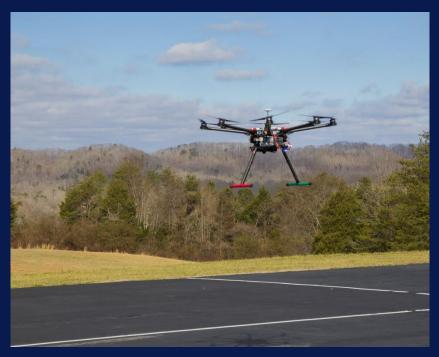
Eight-rotor helicopter capable of carrying up to 4.5 kg payload for 10-12 minutes
