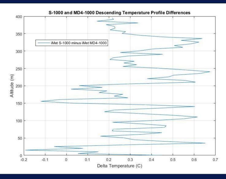
Temperature difference versus altitude (m AGL) for the MD4-1000 and S-1000 descending profiles. Note this data are for the descending portion of the second MD4-1000 profile.
