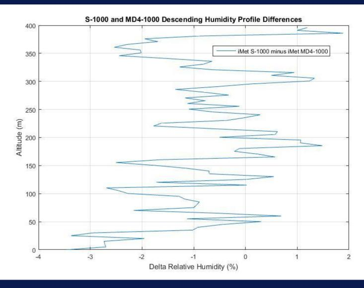
Relative humidity difference versus altitude (m AGL) for the MD4-1000 and S-1000 descending profiles. Note this data are for the descending portion of the second MD4-1000 profile.
