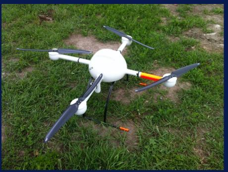
Four-rotor helicopter capable of carrying up to 2 kg payload for 20-45 minutes
