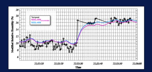
Tempest UAS (black) vs. NSSL Mobile Mesonet time series of Relative Humidity crossing a gust front. The Tempest humidity sensor (RS92), which has a theoretical response time of 0.5 s, detected a large RH increase in just 0.42 s, whereas the NSSL-MM humidity sensor required 17 s for a 90% response to this change.
